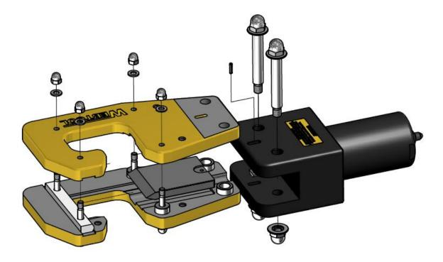
Figure 4 – Removing the blade
