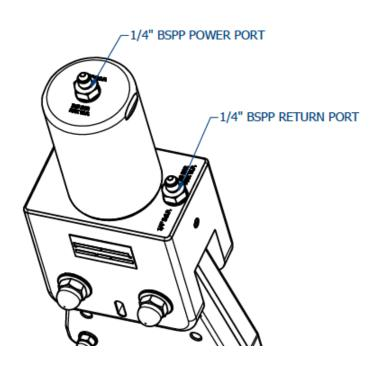
Fig 1 – Hydraulic connection points.
