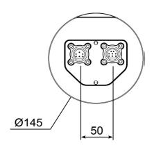
Not to scale, dimensions in mm. Shown with Burton connector. Other connectors are available
